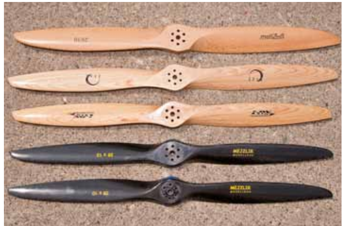
▲ A variety of two-blade propellers were used for testing. The VOX 28x10 and the Xoar 29x10 laminated wood propeller produced the highest static thrust with results in the 58-60 lb range. The Mejzlik 28x12 carbon propellers produced the most pitch speed while still maintaining outstanding thrust. Testing on an airplane will be the true test of which propeller is best for an application.
