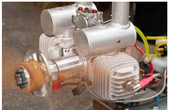
▲ Here is a closeup view of the DA-120 engine at idle, with the Xoar 29x10 laminated wood propeller fitted. Note the optical tachometer/bracket mounted under the lower forward cylinder bolt. This feeds rpm data into the Medusa Power Analyzer Pro system for later analysis.
