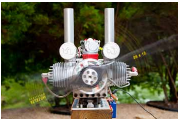
▲ The camera flash freezes the Mejzlik 28x12 carbon propeller while viewed head-on at idle. You can also see how the mufflers fit nicely around the carburetor, leaving enough room for linkages and fuel line, but keeping the overall power plant compact.
